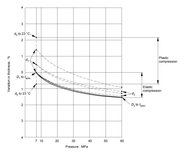
Figure 5 – Elastic compression, plastic compression
